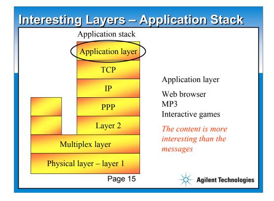
The application layer is the destination for the content from the Internet. The messages controlling the flow of data have all occurred at lower layers, and the content is delivered.
