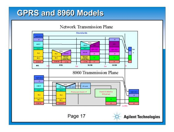
The top picture shows the actual protocol stacks for the data portion of GPRS. On the left is the phone, next is the cell, then the switch, followed by a special switching network to get to the Internet. Finally, on the right, is the Internet itself.
