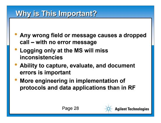
One rule of wireless protocols is that a call must be dropped if anything improper happens. A dropped message is not considered improper. An improper message, or an inconsistent field content can cause this action. It is difficult to troubleshoot this type of problem, as the action of the phone is to suddenly send a disconnect message and leave the link. There are no error messages or trace as to why this happens.
