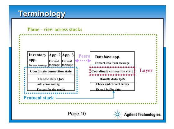
A view like this is called the plane view. It looks down on the layered structure, and shows the stack on each side. The stack is the collection of layers, and a layer is a single entity with specific role in the overall process.
