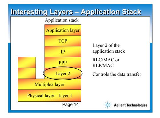
The application stack may take many forms, depending on the nature of the service. Shown here would be Internet access. If a file transfer was started using FTP, the stack would be quite different.
