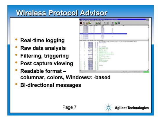
Here is an example of a protocol log on the Agilent Wireless Protocol Advisor. The upper window is the sequence of messages, while the lower window provides the details of the message in blue in the upper window.
