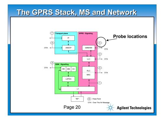
This is a more accurate view of the GPRS protocol stack. Since the layering is symmetrical, this could be either the base station/network, or the handset. In this case, three stacks are shown. The green block is the GSM transmission plane, the pink is the control plane, and the blue is the GPRS transmission plane. Note that the lower layers of the GPRS transmission are handled by the control plane.
