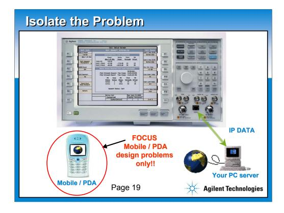
The improved environment is to eliminate all the external switching elements and the Internet. By using local network and Internet emulation, problems can be isolated just to the link to the phone and its internal protocol and application implementation.
