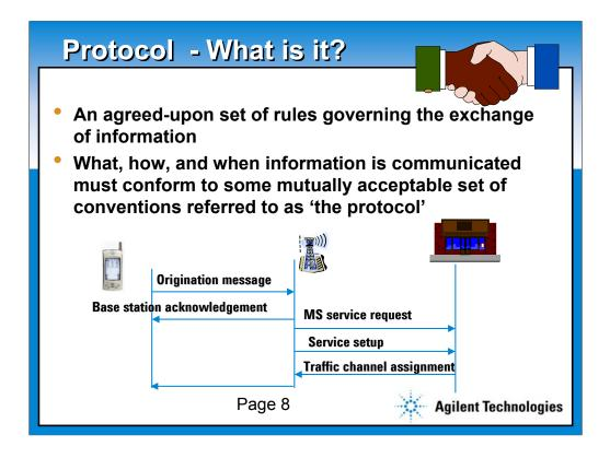
In its simplest form, a protocol is a list of rules on what can be said, and when between network entities. The phone can only talk to a base station, but the base station has two underlying networks, the circuit switched phone network, and the packet switched data network, commonly called the Internet.
