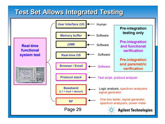
Many different elements of the phone design need testing and validation. Many of these are pure software implementations, and most of the testing can be done before integration. The proper action of these still need to be confirmed with an active RF link and real-world impairments.
