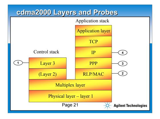
This is very similar to the cdma2000 stack, and the probe locations are shown. As in GPRS, there are probes at layer 3 of the control stack, layer 2 of the application stack, and probes at a few higher layers.
