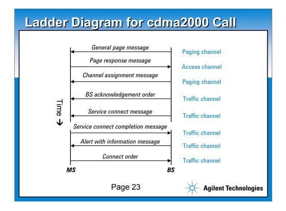
This call processing ladder diagram is from an Annex in the cdma2000 standard. It shows the messages needed for a network initiated voice call.
