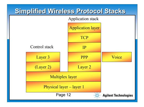
This is a simplified set of stacks. There are really two stacks active when in a packet session. These are the control stack and the application stack.
