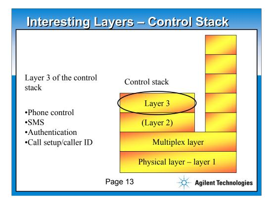
The control stack is where the phone control happens. It is active whether a phone is active or inactive. It may be carried on numerous different physical layers. Typically, there are control channels for this when inactive, and the messages may compete for the traffic channel when active. In modern systems such as cdma2000 and W-CDMA, there may be dedicated channels in parallel to the application. Most of the interest in at layer 3.
