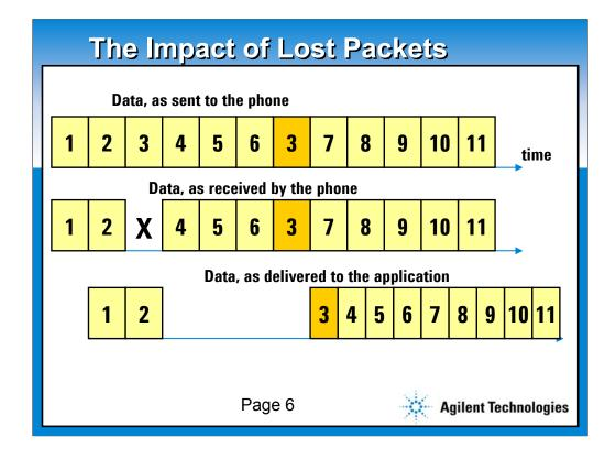
This picture shows the effect of a lost packet. Packet 3 is lost in its transmission. Not shown are the messages between the phone to the network asking for a retransmission. The network is required to put higher priority on re-transmission of a lost packet than on the transmission of a new packet, so the lost packet is sent over the air quickly.
