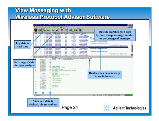
The E6910A's powerful and full-featured protocol analysis capabilities are provided by the Windows executable Wireless Protocol Advisor software running on an external PC, connected to the instrument via the LAN port. Includes:
